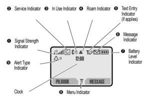
Signal Strength Indicator: Shows the strength of your phone's connection with the network.
